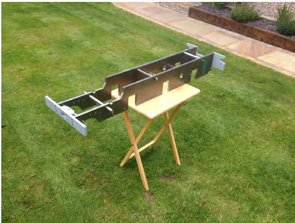
Frames buffer beams and stretchers on a nicely cut lawn!
