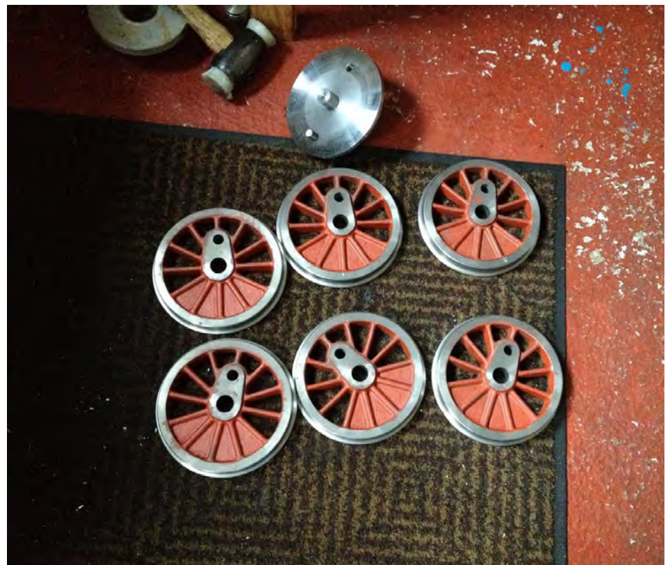
Drivers machined and crankpin holes reamed (note lathe holding jig)
